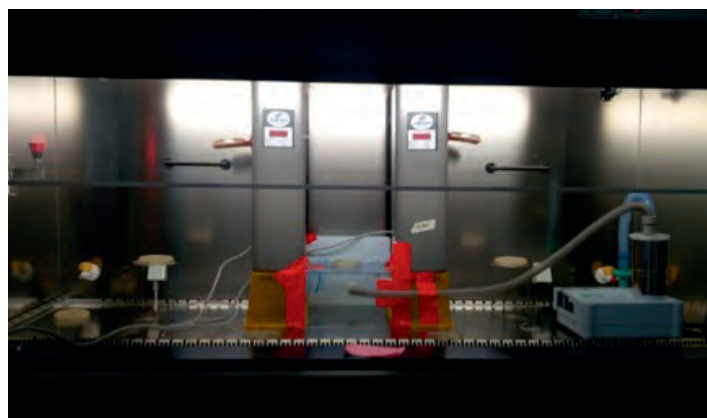
Photo 1: Test set up Air 160, vaporiser and settling plates
